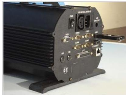
Numerous standard ports are compatible with most standard peripheral equipment.
