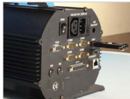
Numerous standard I/O ports are compatible with most peripheral equipment.
