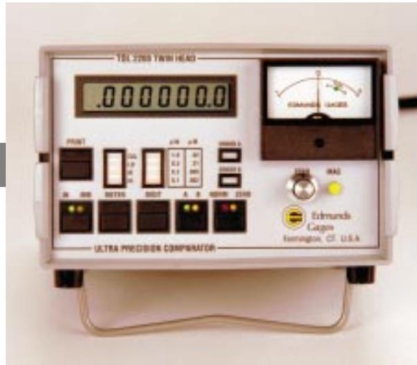
***For calibrating the entire range of gage blocks at a resolution of one-tenth of one millionth of an inch — the Edmunds Gages Ultra-Precision Twin-Head Gage Block Comparator***
