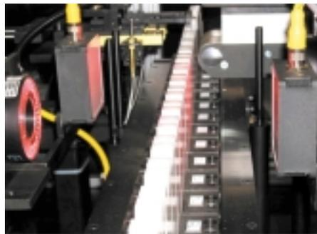
2) Parts handling components place parts in vee blocks on an indexing conveyor. Valves are comparatively viewed and measured with high resolution cameras. They detect size by thousandths of an inch, not number of pixels, to determine "accept" or "reject" status.
