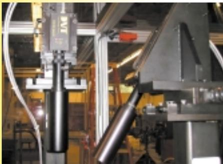
1) Flexible gage measures a family of valve guides at 10,000 parts per hour. Lengths range from 1.25" to 3", diameters from .375" to .625". The features checked were chamfers on both ends, length, chipped faces, the presence of a ground surface, OD, and I.D.
