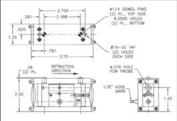
Reverse, normal spring air retract for cartridge probe 5312090
