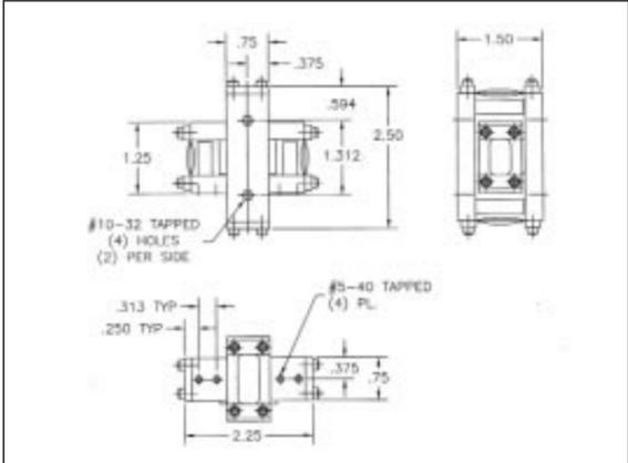
X-Y combination package for cartridge probe 5312070
