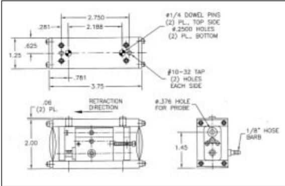
Forward normal spring, air retract for cartridge probe 5312023
