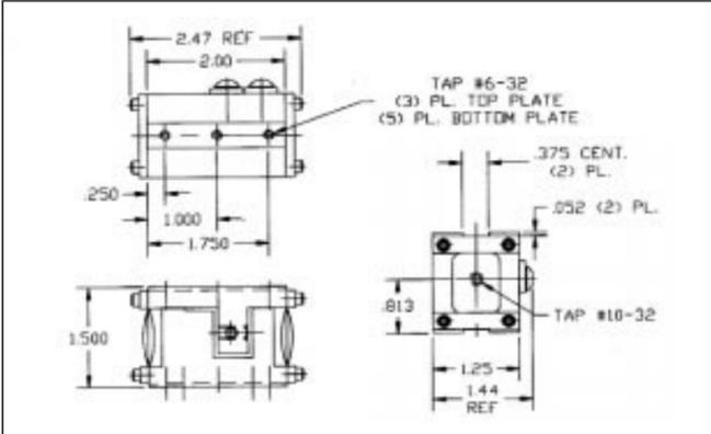
Aluminum with integral LVDT gage probe 5010100
