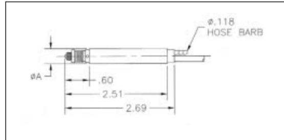
3/8" dia., .080" range, 8' cable, 4-48 thread ..... 15144C-38-8-PE
