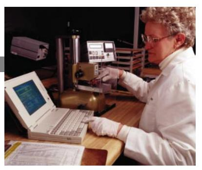
Gage block calibration is one of our specialties. Suited to all users of square or rectangular gage blocks in all grades. Measurement and reporting conform to ASME/ANSI B89 1.2M and ISO 3650. Using progressive equipment and experienced metrologists, you get accurate, fast, and economical service. Many customers also take advantage of our automatic gage block replacement program.
